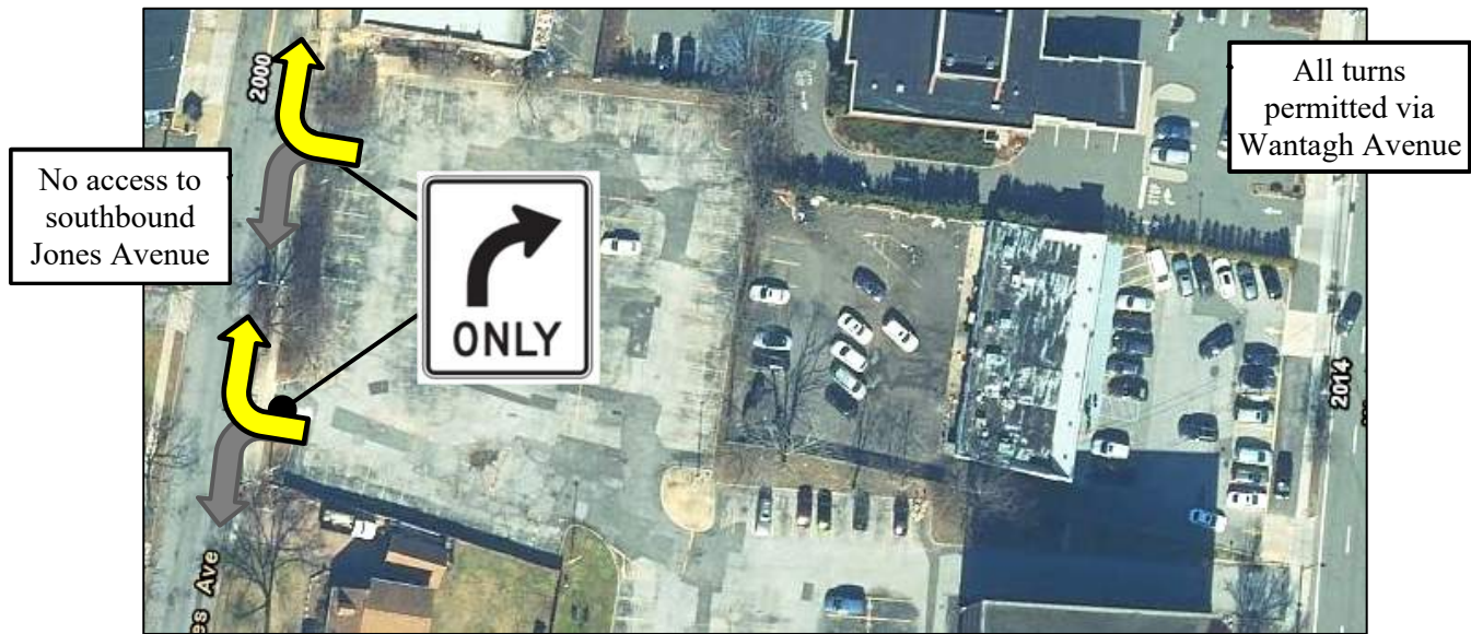
Figure 3: Proposed Site Access Permitted Turns
